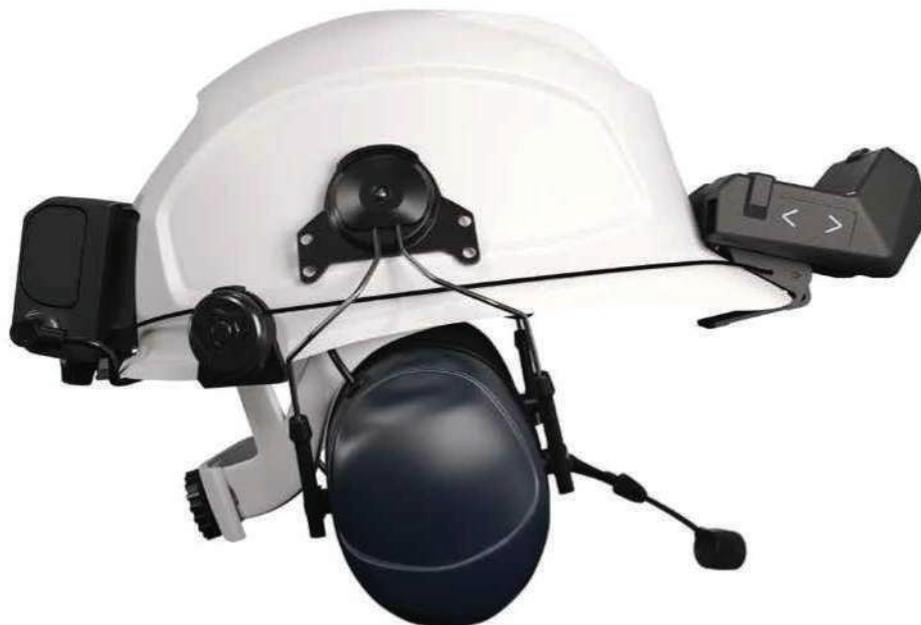
Kiber 3S Kit empowers field workforce with a wearable hardware for remote assistance based on AR technology: a head-mounted device with a unique binocular visor, an HD video camera, a high performances set of headphones/microphone and a 12GB local storage to store documents locally. Designed to perform and satisfy the real needs of remote working operations.
