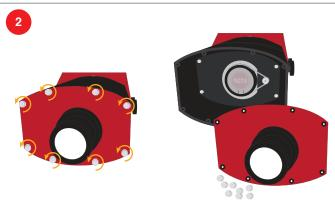
Remove the front cover (with the projection lens) by removing the eight screws holding it in place.
