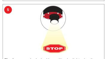
The focus can be locked in position by tightening the retaining ring on the focusing lens onto the projector body. Note that there is a rubber O-ring to prevent the retaining ring from damaging the projector.
