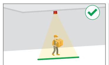
**IDEAL MOUNTING** Unit should be mounted perpendicular to the surface exactly midway of the desired projected length. E.g. if the unit produces a 20ft line from the defined mounting height, the unit should be mounted 10ft away from the start of the line
