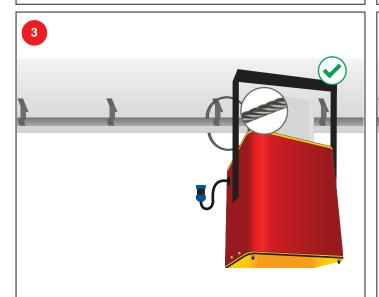
Finally, be sure to loop the included steel safety cable through the eyelet on the back of the Virtualine™ LED SWITCH and around the nearest secure object, pipe, or rail. This is to prevent injury in the unlikely event that the primary mount fails.
