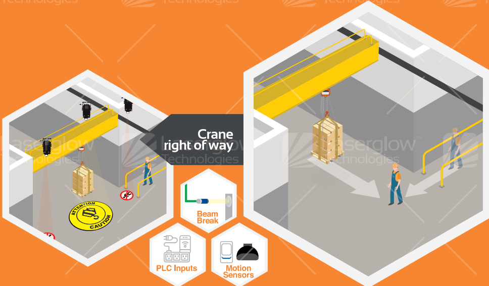
When the load is approaching, signs will be display indicating the upcoming hazard above.
