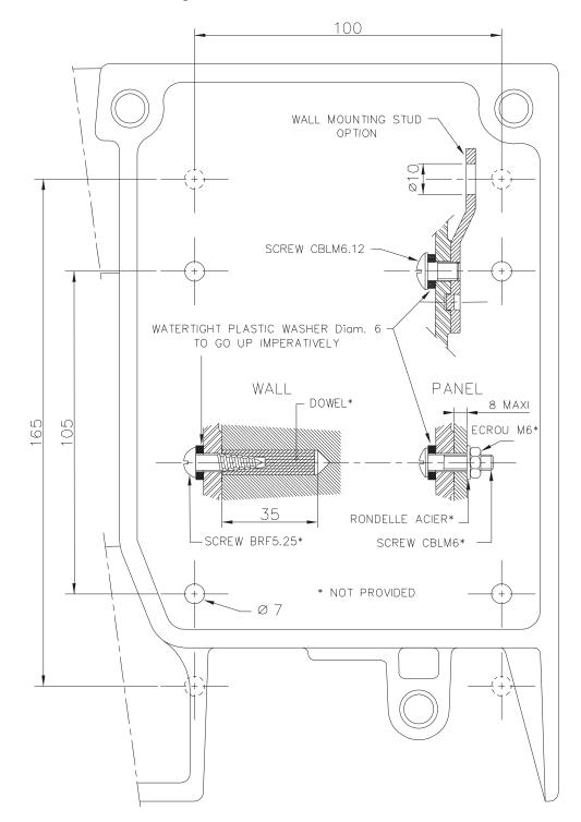
Tailoring the diameters of cables with diameters of knockouts (Ø10 to Ø13 Maxi) and tighten them correctly.
