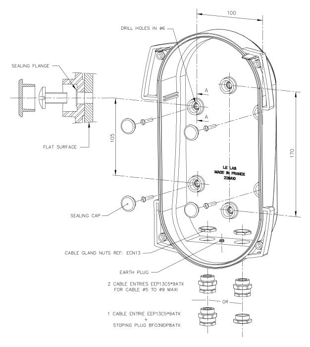
Adjust cable diameters to the diameters of cable glands (Ø 5 to 9 Max) and tighten properly.
