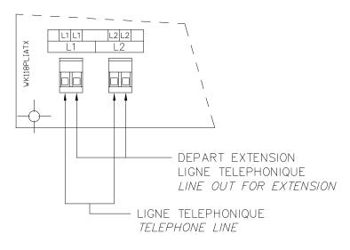
Connect the telephone line terminals L1 and L2. Connect ground.
