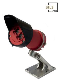
The **IPES-IR/UV** is constructed in an explosion-proof housing for use in hazardous (classified) locations and meets the industry certifications and requirements of Class I, Division 1, Group B, C & D, T5.
