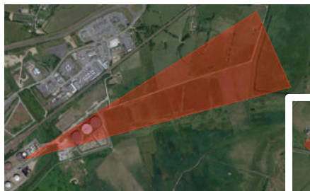
Multiple tanks roof monitoring using 1 or 2 cameras
