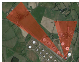
Multiple tanks roof monitoring using 1 or 2 cameras
