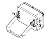
POSITION STIRRUP TO PREFERRED ANGLE AND SECURE USING REMAINING M6 SREW, SPRING-WASHER AND NUT (ITEM 9)
