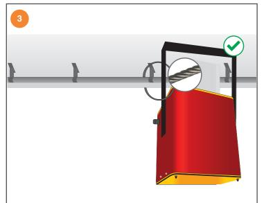
Finally, be sure to loop the included steel safety cable through the eyelet on the back of the Virtualine™ LED EDGE and around the nearest secure object, pipe, or rail. This is to prevent injury in the unlikely event that the primary mount fails.
