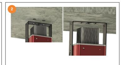
Then affix the Virtualine™ LED EDGE to your mounting surface using hardware designed for that type of mounting surface (drywall anchors for drywall without a stud, concrete screws for concrete). Once the fixture is in place, clear any dust or debris out of the rear heatsink area before powering on the fixture.
