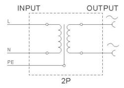
Transformer is equipped with a external bonding point which can be used if preferred. Using the bonding point is not mandatory, since the PE conductor is connected through the supply cable.
