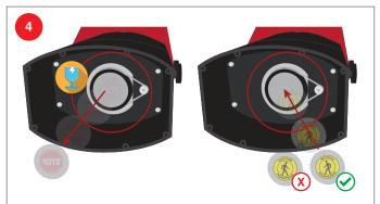
Carefully remove the old image template and replace it with the new image template. The image template should appear to be backwards or mirrored when looking into the front of the projector.
