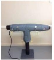
protect devices from environmental impacts like precipitation, icing, wind load capacity, direct solar radiation, high temperatures, corrosive liquid and to reduce heat loss. The light-weight construction of these removable enclosures means they are selfsupporting which eliminates the need for costly support frames or brackets. MATTCOLD are custom made to the dimensions of the instrument. accounting for any supports and
