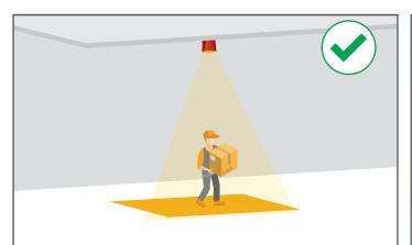
**IDEAL MOUNTING** Unit should be mounted perpendicular to the surface exactly midway of the desired projected length. E.g. if the unit produces a 20ft walkway from the defined mounting height, the unit should be mounted 10ft away from the start of the walkway.
