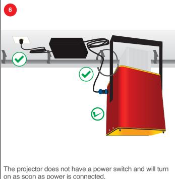
**NOTE:** When installing the power supply, do not add cable extensions between the power supply and the light fixture. The length of cable between the power supply and fixture should be as short as possible (6 feet maximum, 3 feet or less recommended). Any extensions required to bring power to the projector should be added on the AC side of the power supply.
