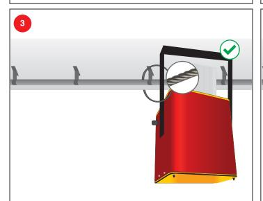
Finally, be sure to loop the included steel safety cable through the eyelet on the back of the Virtualine™ LED FILL and around the nearest secure object, pipe, or rail. This is to prevent injury in the unlikely event that the primary mount fails.
