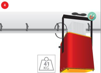
If you purchased the magnetic mount accessory, your mounting bracket will already have the magnets installed. Simply stick the magnets to the desired surface and loop the included steel safety cable around the attachment point to prevent the fixture from falling if the magnets fail. The magnets hold with approximately 90 pounds (41 kg) of force.
