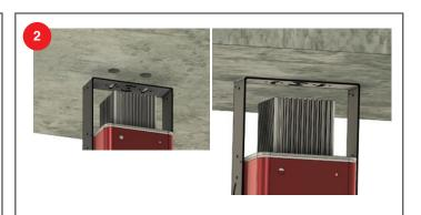
Then affix the Virtualine™ LED FILL to your mounting surface using hardware designed for that type of mounting surface (drywall anchors for drywall without a stud, concrete screws for concrete). Once the fixture is in place, clear any dust or debris out of the rear heatsink area before powering on the fixture.
