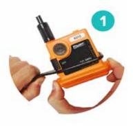
Remove the sMRT AU10 from the PFD, as per manufacturer's instructions and lift the RESTRAINER TAB up and over the ARMING SWITCH.
