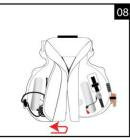
Fold the right side bladder lobe (as worn) at the centre front edge once to the outer edge.
