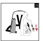
Fold the bottom part of the left side bladder lobe (as worn) back towards the lower edge of the cover; tucking the surplus underneath.
