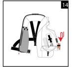
Fold the bottom part of the left side bladder lobe (as worn) away from the lower edge of the cover.
