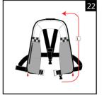
Using the zip slider, pull the zip all the way from the bottom centre front up to the top back neck and ensure that you pull it all the way to the end of the zip under the velcro and fasten the velcro securely back over the end.
