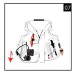
Fold the bottom part of the right side bladder lobe (as worn) back towards the lower edge of the cover; tucking the surplus underneath. Ensure the beacon is positioned
