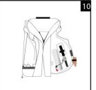
Position the inflator pull cord and handle out of the back slot in the cover ensuring that it hangs down freely at the back.
