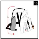
Then pull the zip slider all the way back down again to the bottom centre front. The zip should now be completely closed on this side and the bladder, beacon and antenna securely inside the cover. Fasten pull the dot press-stud from zip slider onto the back of the cover. Make sure that both indicators on the inflation system are clearly visible through the window on the back and are fully green.
