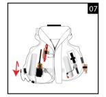
Fold the bottom part of the right side of the bladder lobe (as worn) back towards the lower edge of the cover ; tucking the surplus underneath.
