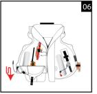
Fold the bottom part of the right side bladder lobe (as worn) away from the lower edge of the cover.
