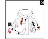
Fold the bottom part of the right side bladder lobe (as worn) away from the lower edge of the cover.
