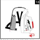
Fold the left side bladder lobe (as worn) at the outer edge so that the buddyline is tucked away to the back.
