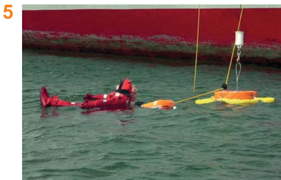
The person(s) can be pulled to the floating rescue disc and can hold tight.
